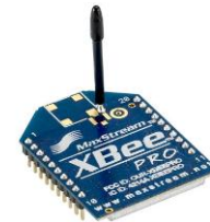
Gambar 9. Modul Wireless Xbee Pro (IEEE 802.15.4) [7,10]
